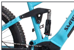
140mm / 120mm Front & rear travel air coil suspension
